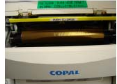
Press on the 'push to open' yellow strip.
