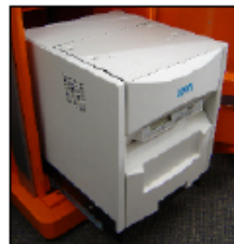
Push the paper tray in to the unit.
