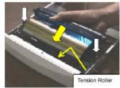
Install the Ink Ribbon on the tray.
