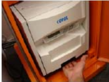
Pull the black tray out from inside kiosk with printer on it.
