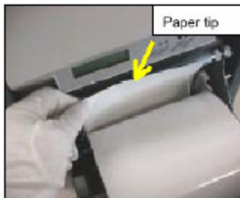
Engage the pressure roller again.
